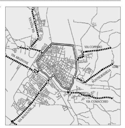
Although relatively short (some 3 km.), the Pontegradella link is a good example of a outer urban greenway, since it is used daily by Pontegradella inhabitants who come to Ferrara to work or study. The path, 2,5 metres wide, has been asphalted and is lit by street lamps situated at 15 metre intervals. Two design footbridges cross the canal to link the road and adjoining residential area. The greenway is separated from the canal by a 2,5 m strip of land which is used by maintenance vehicles.
