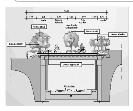
A pedestrian/cycle axe will be established on the covering over the railway line (Source: City of Rome).
